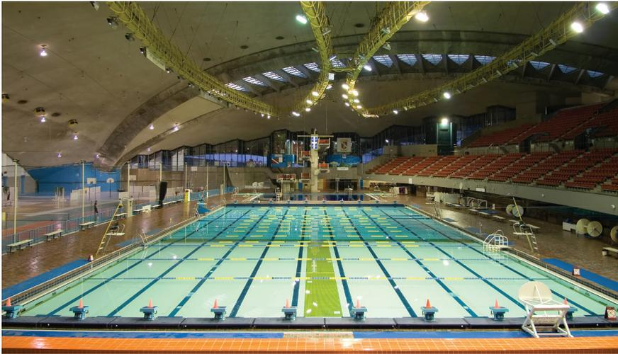
*Healthy and durable pool spaces require proper air distribution to all space micro-zones. Zones shown here include swimming, deck, and elevated spectator areas, and exterior-facing glass, wall, and roof areas.*
